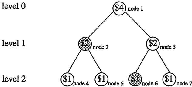
Figure 3. A binary tree for a divisible coin worth \$4.00, with a minimum unit of \$1.00. A \$3.00 payment can be made by spending the shaded nodes. Node 1 cannot be used in a subsequent payment because it is an ancestor of nodes 2 and 6. Nodes 4 and 5 cannot be used because they are descendants of node 2. Node 3 cannot be used because it is an ancestor of node 6. Nodes 2 and 6 cannot be used more than once, so node 7 is the only node which can be spent in a subsequent payment.
